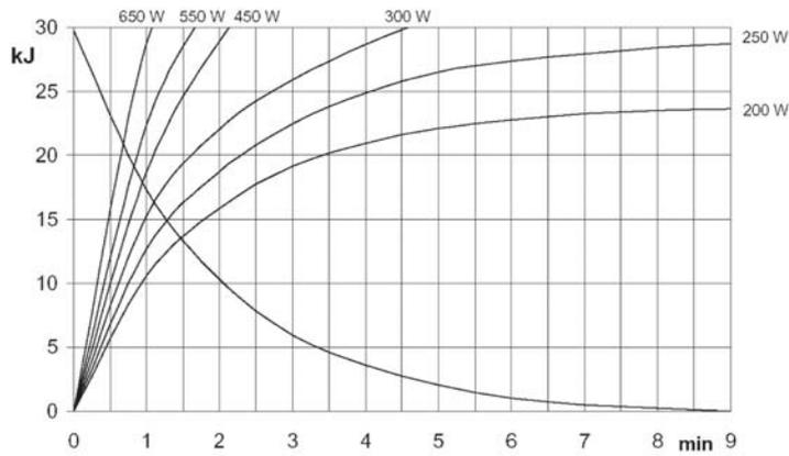
**Figure 7-3 Single Load Chart of the X-ray Tube**
