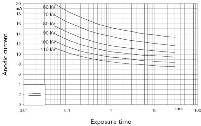
**Figure 7-4 Filament Emissions of the X-ray Tube**
